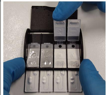
7. Close the lid of the Test Chip holder and insert the chips into the Instrument.
