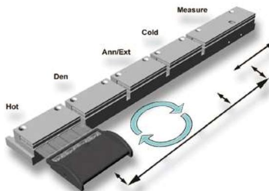
**Figure 1. Thermal blocks of the GenomEra Instrument. Each block serves a specific function in the PCR thermocycling sequence: Hot, Denaturation (Den), Annealing/Extension (Ann/Ext), Cold and Measure.**
