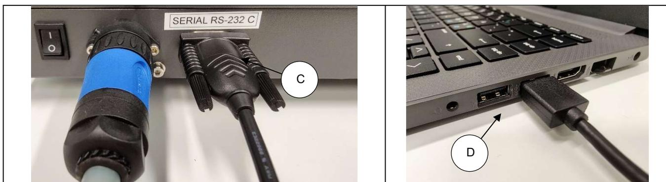
5. Connect the printer to the USB hub using the USB A-to-B cable. Also connect the printer to a power outlet.
