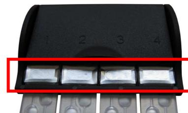
Ensure that all cables and cords are tightly connected and all the accessories work as normal. Ensure that the chip holder (especially the narrow support structures in the front) is intact and is stable when put on a flat surface. Discard all old, bent, or broken chip holders.
