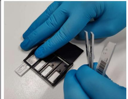
5. Add 35 µL of prepared sample per Test Chip. Insert the pipette tip into the sample opening in an upright position and ensure that the tip is firmly in place in the opening. Take care to avoid bubbles forming.
