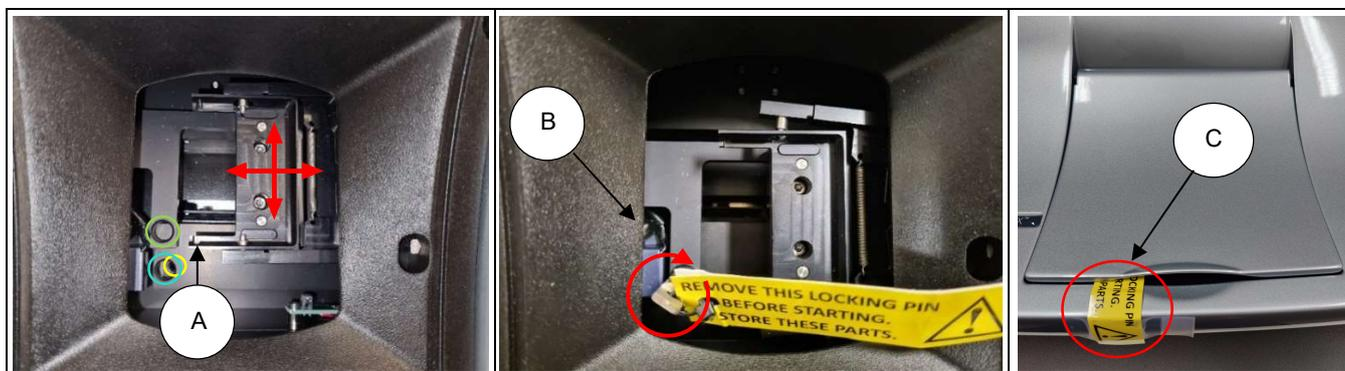
**!** **Note:** The Instrument should not be transported without the Locking Pin fastened. Contact Technical Support if the Locking Pin or the attached warning label is missing.
