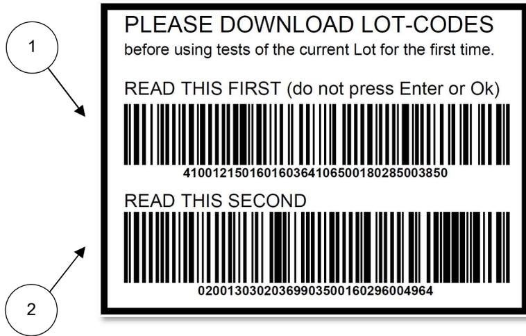
3. Read the first part of the barcode (1) by moving the barcode reader from top-to-bottom.
