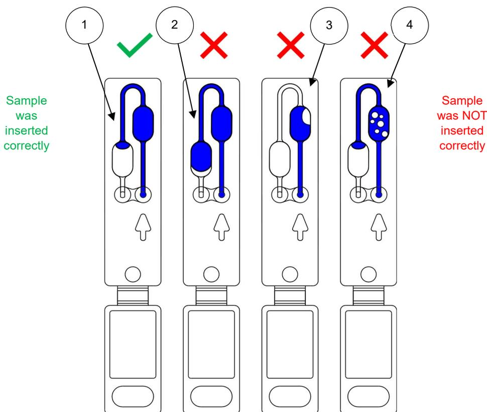
Always discard a Test Chip with excess sample volume (2), insufficient sample volume (3) or visible air bubbles (3, 4) and restart Test Chip preparation with a new aliquot of sample. The Rehearsal Chips provided with the System can be used for pipetting rehearsal.
