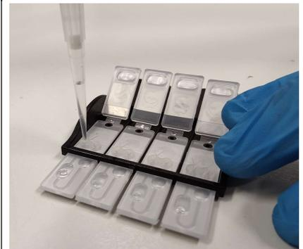
6. Close the lid of each Test Chip **individually** by pressing the lids firmly over the sample openings.
